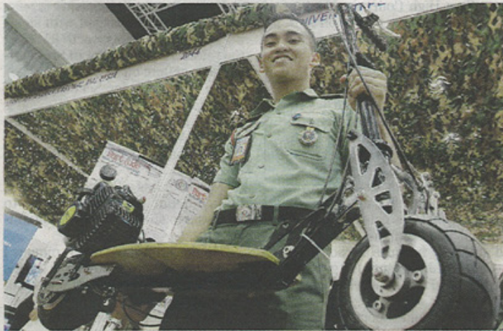
The 'Port-Ride' motorised scooter can be folded up and carried around in a haversack.
